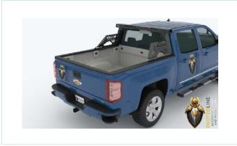
SOLDIER ROLL BAR ADD STYLE AND FUNCTIONALITY TO YOUR PICKUP TRUCK. THEY AFFIX TO YOUR TRUCK BED AND ALLOW YOU TO MOUNT ADDITIONAL LIGHTING AND GIVES A MORE RUGGED APPEARANCE. THE PRODUCT IS SHIPPED DISASSEMBLED, MAKING IT EASY TO TRANSPORT AND HANDLE
